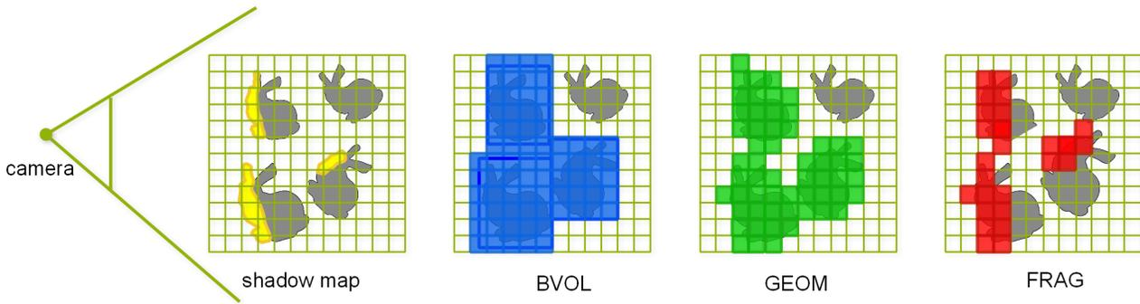
**Figure 2:** Visualization of different receiver masks. On the left there is a light space view of the scene showing surfaces visible from the camera in yellow. On the right three different receiver masks are shown. Note that the invisible object on the top right does not contribute to any of the receiver masks.
