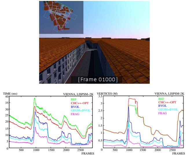
**Figure 5:** Dependence of the frame time (bottom left) and number of vertices (bottom right) for a walkthrough of the Vienna scene and different shadow computation methods. Note that the walkthrough also includes viewpoints located above the roofs. Such viewpoints see far over the city roofs (top). In this comparison the FRAG method achieves consistently the best performance followed by the GEOM+BVOL method.
