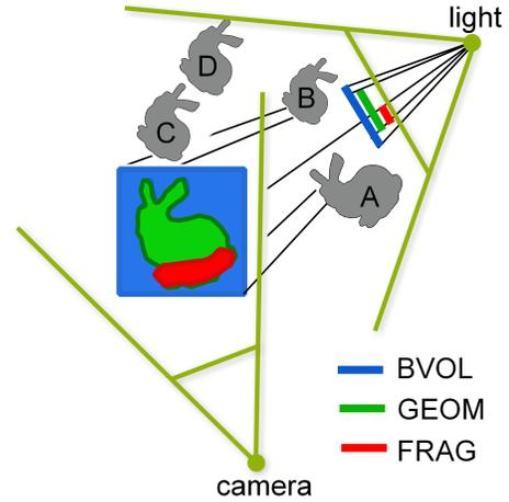
**Figure 3:** 2D illustration of the culling efficiency of different masking strategies. The figure shows an example of the scene with a shadow receiver object and different types of shadow receiver masks. Object A is always rendered as it intersects all masks, object B is culled only by the FRAG mask, C is culled by depth test (occluded by B) and by the FRAG and GEOM masks, and finally D is culled by all types of masks.
